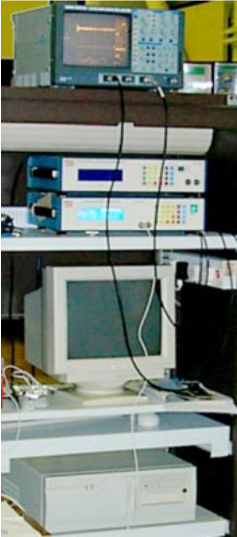
Fig. 2. Photograph of the oscilloscope, amplifier, pulser/receiver cable, and mainframe computer.
